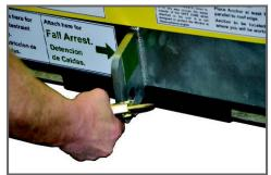
Your lanyard can connect to either the fall-restraint or the fall-arrest.
